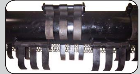
3 - 8" Long cupped blades mounted on one shaft for easy changing
