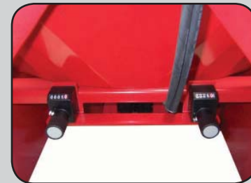
Right and left band shutter opening dials, hydraulic off and on from the tractor
