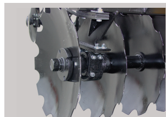
Trunion mounted bearings absorb more shock loads & improve bearing life
