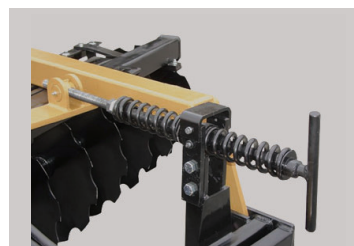
Self-leveling spring cushioned with hand crank
