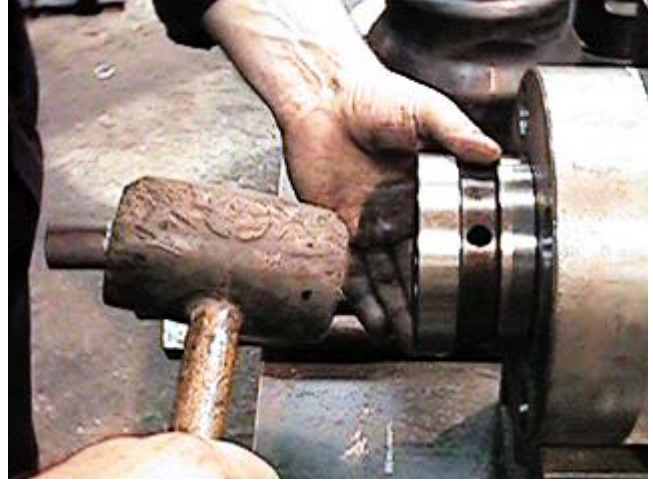
Carefully tap the lower cylinder liner into the main cylinder with a rubber or hide hammer.
