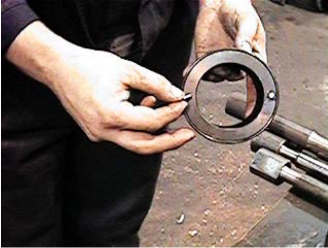
Insert the locator keys that are used to align the cylinder liners.
