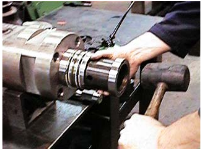
Install the seals and packing to the upper cylinder liner. Align the upper and center cylinder liners then use rubber or hide hammer to install the upper liner.
