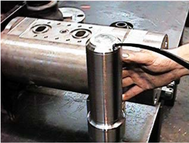
Apply working oil to the piston.
