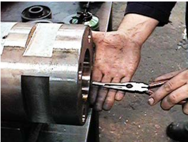
Insert locator keys into center cylinder liner.
