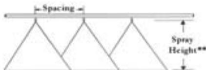
\*\*Adjust spray height in the field to overlap approximately 30% of each edge of pattern.
