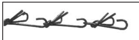
MINIMUM ACTION Tines up in smoothing position
