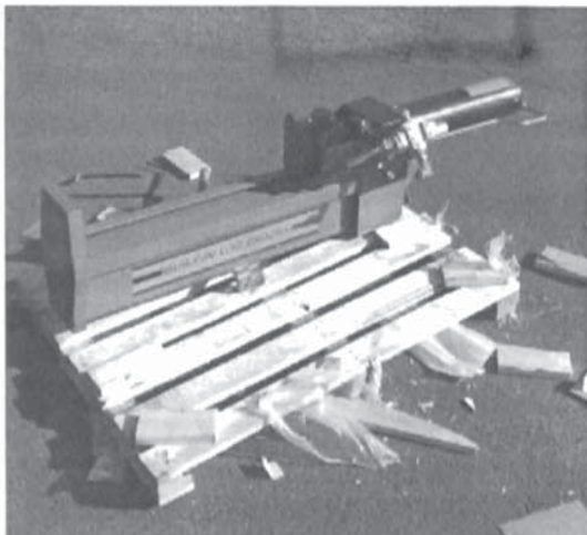
Cylinder pushed all the way back and stripper plate attached (see steps 6 - 7, pg. 8).
