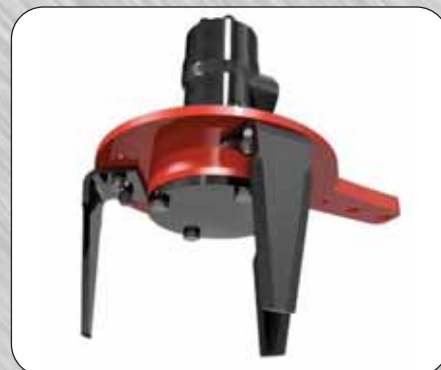
Hydraulic driven power harrow w/3 replaceable blades
