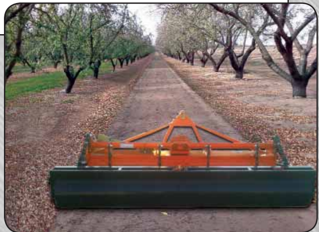
Optional roller cleans, fills and rolls orchard floor
