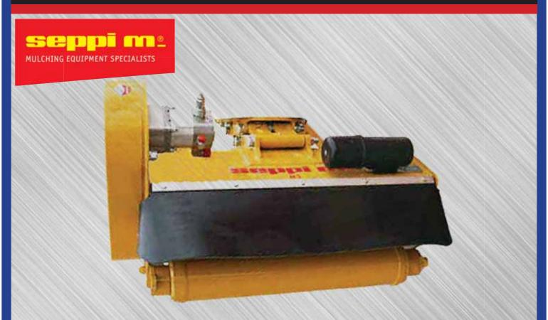
These Flail Mulchers are ideal for grasses and brush that are difficult to reach, like edges of roads and riverbanks. These units shred material up to one inch in diameter. The Mulchers are very productive even with the low hydraulic power required. The hood is made of wear resistant steel. The adjustable rear roller is reinforced and the floating mount adapter are standard equipment. These mulchers are strong, yet light weight for better control. Available cutting widths of 33 & 41 inch.
