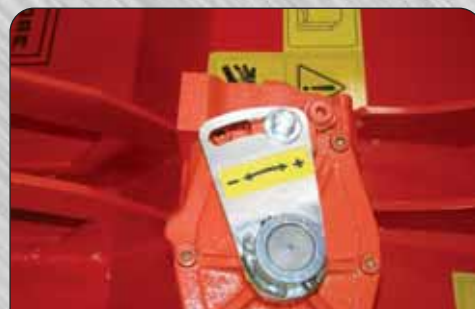
Piston Motor w/Adjustable Gallons Per Minute
