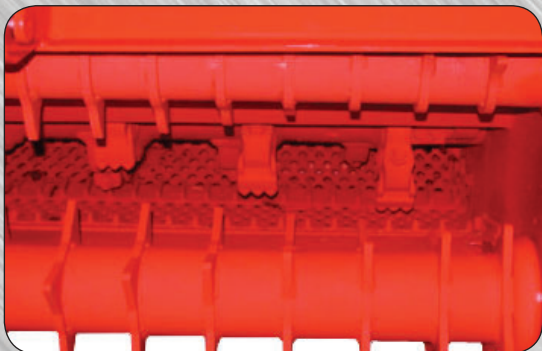
Knives, screen, re-cutter bar and lower pick-up rotor
