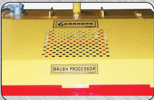
Vented panel over the oil cooler fan for protection
