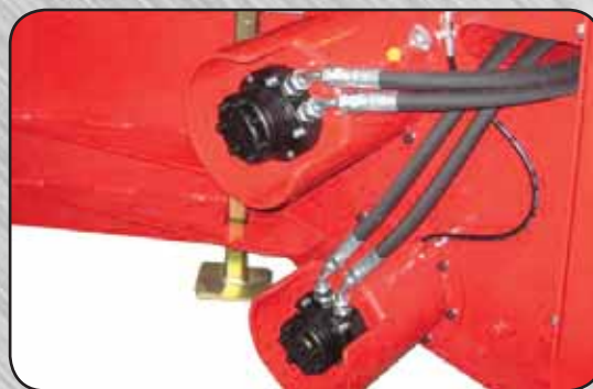
Two hydraulic motors power the feed rotors with protective casing
