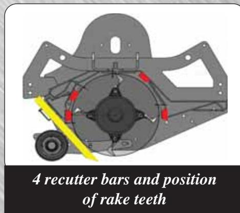
*4 recutter bars and position of rake teeth*
