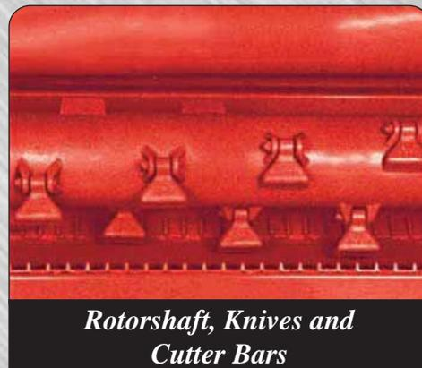
*Rotorshaft, Knives and Cutter Bars*
