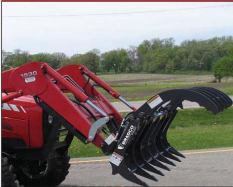
The aggressive tine shanks root out objects below ground level. The wide grapple opening allows for gathering a large amount of brush and debris. The hydraulically operated grapple locks the material in place and stabilizes it for transport.
