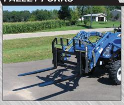
High strength lightweight frame for large 2300 pound pay loads. Open guard for excellent visibility. Patented load retention ring. Class II ITA forks with positioning lock pin.
