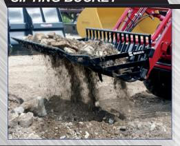
Designed to collect rocks and debris, allowing soil to sift through. Rake design allows for fast clean-up, ground leveling and gathering materials away from buildings and obstructions. Leave the dirt and pay less at the land fill!
