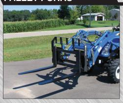
High strength lightweight frame for large 2300 pound pay loads. Open guard for excellent visibility. Patented load retention ring. Class II ITA forks with positioning lock pin.
