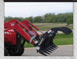
The aggressive tine shanks root out objects below ground level. The wide grapple opening allows for gathering a large amount of brush and debris. The hydraulically operated grapple lock the material in place and stabilizes it for transport.
