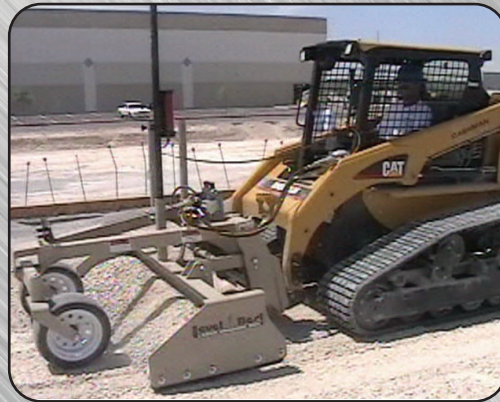
Caterpillar track loader and Para-Level grading scraper at work.
