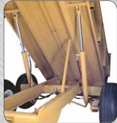
Dual Hydraulic Cylinders and Safety Lock Bracket
