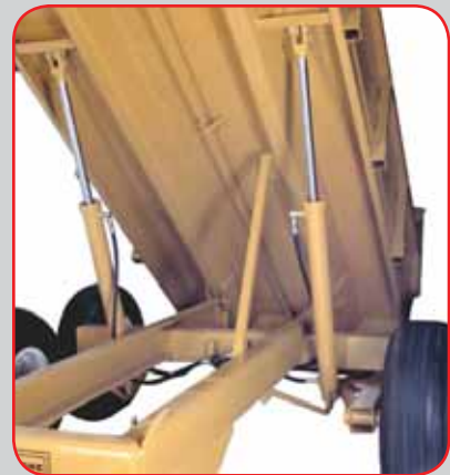
Dual Hydraulic Cylinders and Safety Lock Bracket
