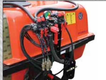
Control Valve and Hydraulic Hoses
