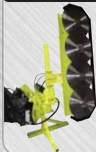
The **L.E.M.® Sawhead** module was designed for mounting to many different types of equipment such as: tractors with front loaders, skid steer tractors, compact excavators etc. This Sawhead comes with a heavy 4" square beam for mounting. The body of the Sawhead is made of rust proof anodized material which is light weight, but stronger than steel. This housing module will not deform.
