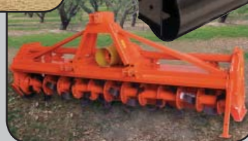
T Tiller with adjustable rear roller
