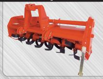
These medium duty "N" Series Tillers feature a smooth running, all gear drive system. Powered through a heavy 70 horsepower gearbox to an all gear final drive. The tilling action provides a uniform mixture throughout the cultivated depth. Producing loose textured soil that holds moisture and reduces erosion.
