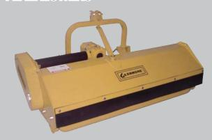
This Gearmore SLE Series flail mowers were developed for mowing grass and light weeds with side slicing Y blades. All models are also available with finish mowing cupped "ducksfoot" blades for mowing grass. Standard features include ASAE quick attach 3-point hitch, low profile design, center mount or offset, adjustable rear roller and many more. These flail mowers were designed to achieve fine shredding in parks, schools, and golf courses.
