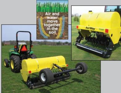
This is a fast, effective, low cost method to keep the soil surface open and minimize compaction without disrupting use of the turf area. As surface compaction is a continuous problem, caused by both use (foot traffic) and maintenance (mowing), venting aeration should be scheduled as often as possible to be effective. *AerWay's* complete line of *Turf Aerators* feature 5 different tine rotors to handle your exact requirements. The polyethylene built-in ballast tanks, when filled with
