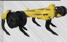
The GE Series of 3-point hitch mounted Rippers was designed for extreme duty subsoiling. The Rippers have A.S.A.E. quick hitches for Cat. 3 and 4N tractors. The shanks are "L" style, 1  $\frac{1}{2}$ " thick by 36" long. Optional gauge wheels are available in single or dual steel wheels and single or dual rubber tires.
