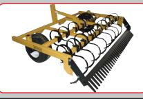
The *AC Series* of Arena-combs were developed for the highest quality arenas that usually have a decomposed granite or ground rubber base under approximately 4 inches of quality sand. If the base material is disturbed the arena will be damaged, thus two large adjustable 8" wide floatation gauge wheels are mounted in the front. Then the two rows of vibrating S-tine shanks loosen and aerate the soil. The special 3/4" thick steel comb levels, gauges the depth, lightly compacts, and combs the sand.
