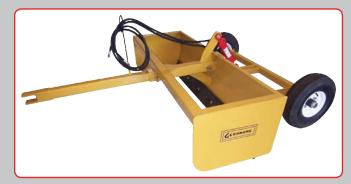
For larger ranches our *CD5*, 6 & 7 foot drag scrapers are a great road maintenance tool. Also good for building arenas, it perfectly grades and levels base material and sand. The scrapers are hydraulically controlled from the seat of your tractor. The floatation gauge wheels allow you to set the cutting edge to build and maintain roads using the same concept that is used in building highways today.
