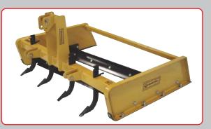
Our *Grading Scrapers* are an excellent implement for access road maintenance. The dual blade, flow through action cuts out high spots, fills holes, and moves material from the outer edge of the road toward the center, thus achieving a smooth finished road. These compact scrapers are available in 5, 6, & 7 foot. This is an extremely easy tool to operate.
