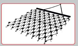
This is a low cost popular way to finish groom an arena. These harrows smooth rough spots, fill in holes and incorporate moisture. The popular sizes are 4, 5, 6, and 8 foot widths. If you plan to keep your harrow close to the arena, this is an acceptable tool.
