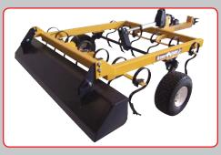
The *Arena-Vator Junior* is a complete self contained towable implement that can be operated by almost any vehicle. The tilling depth is controlled by an electro cylinder operated from the vehicle seat. The unit is also available with a manually operated turnbuckle. The two rows of "S" time shanks vibrate in a circular motion when contacting the ground, thus loosening and cultivating a large area around the shank points. The adjustable rear finishing box contains and levels out the soil.
