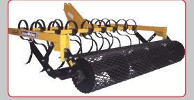
The *AV Series* of Arena-vators were designed to renovate and condition horse arenas and tracks in a single pass. The machines consist of two rows of vibrating S-tines to loosen and cultivate the soil, an adjustable bar to level the soil and a rear roller to help gauge the depth. The rear roller is available with mesh or spiral rod, depending on the finish you desire.
