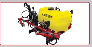
Our *Model UTL-40-5* sprayer with 40 gallon poly tank will handle most spraying projects around the ranch. The simple electric pump is powered by the battery on your towing vehicle. This diaphragm pump was designed to handle herbicides. Standard equipment includes handgun with 25 feet of hose and boom with 100" coverage.
