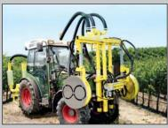
The patented COLLARD system achieves leaf removal by a flow of low pressure air produced by a 3-point hitch, PTO driven air compressor. The air is blown through the leaves at fruit level by adjustable rotating defoliating heads. This rapid pulsing air literally shakes the leaves from the foliage and rattles the caps free from
