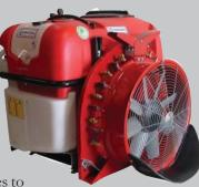
isolate it from vibration and stress. The gearboxes have a neutral position, which shuts off the fan during handgun or boom work.
