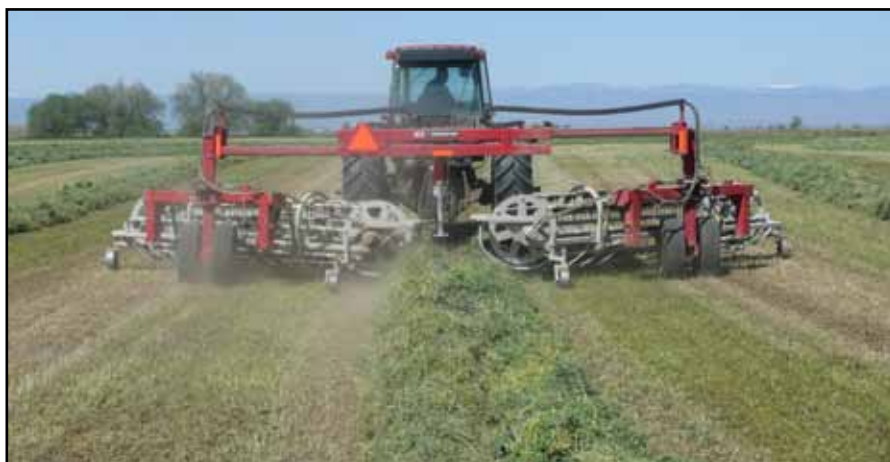
Fig. 14 BASKETS LOWERED AND RAKING
