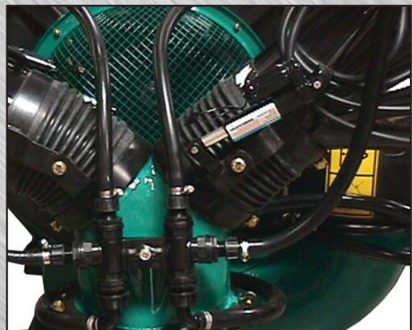
Optional Electro Cylinders To Adjust Nozzles For Different Plant Heights
