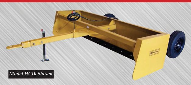
The "HC" High Capacity Series of Drag Scrapers feature heavy, large side plates - ½" thick. These side plates are 30" high by 40" deep, thus allowing for dragging and depositing large amounts of material. Like the "AP" series, the beam tongue extends to the rear moldboard and is held in place by a 5" x 5" heavy gusseted tube. The new axle assembly is built with 4" x 2" tubing. The larger dairies and feedlots find these scrapers best for their operations.
