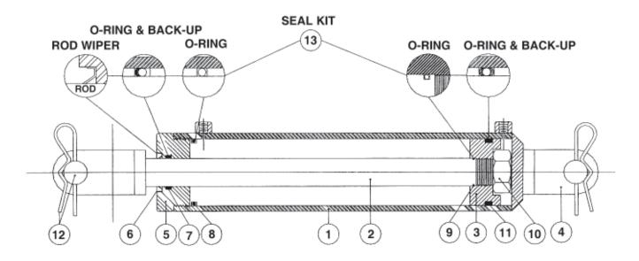
"This Cylinder is Round Barrel - Non Tie Rod Design"
