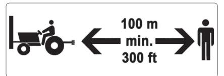
DANGER: This machine has dangerous moving parts. Keep a safe distance from the tractor and implement.
