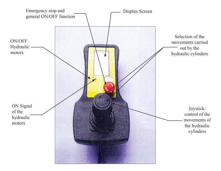
To carry out a movement of a hydraulic cylinder, operate the joystick by tilting it towards one of the 4 directions following the desired cylinder movement.
