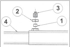
Check the plastic plug for wear, by removing the central screw. Replace it if necessary. (**Use only original spare parts - see table**)
