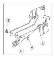
Loosen the bolt (3). Remove the bolt (4) and the nut (5). Give the angle chosen of the vertical cutting element. To put the bolt (4) in the nearest hole of the bar (6). Tighten the bolts (4) and (3).
