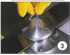
Blades RH operate in CLOCKWISE (No groove on the flange)
