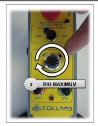
**Step 2:** Turn speed knob to the right which is maximum speed
