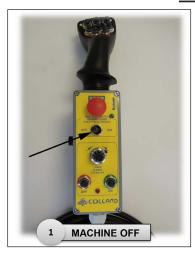
Step 1: Turn machine off at control box
