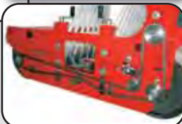
Chain/Sprocket Rear Roller Drive
