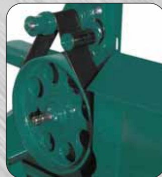
Power band fan speed up system with built-in overrunning clutch
