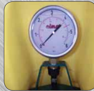
Large 3" dia. glycerin filled gauge, easy to see from tractor seat
