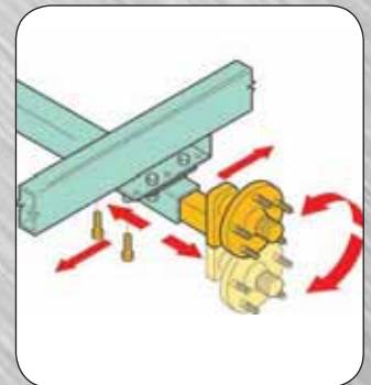
Wheels adjust up or down, in or out, front or rear to obtain best balance and clearance
