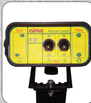
Electro valve controls to operate on, off, left, and right spraying
