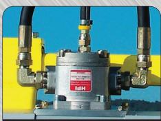
Hydraulic motor provides high powered transmission to blades
