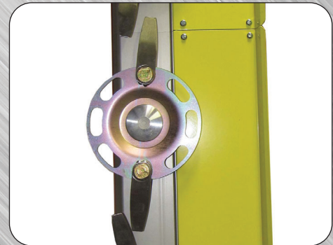
Double edge knives overlap for cleaner cut
