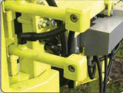
Optical cells that are for automatic opening and closing cutting heads
