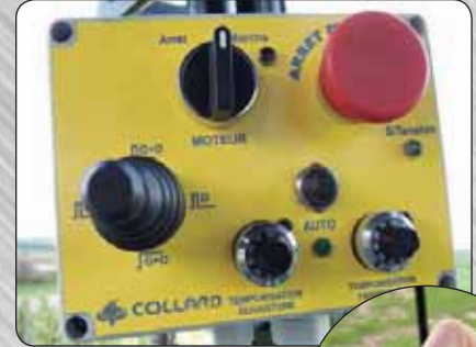
Control panel and hand switch for manual override optical cells (electric eyes) allows for automatic retraction on all types of posts
