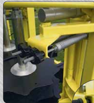
Trellis post protection, also includes hydraulic dampers
