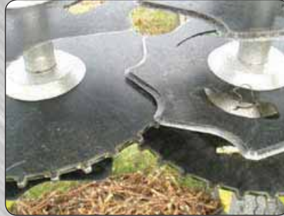
Cutting blades and notched discs for clean cuts and trellis post protection.
