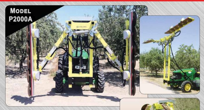
The *COLLARD Hedger* is a total pruning system for orchards. Features an adjustable pruning system to hedge, top and skirt orchards. Allows growers to maximize production and reduce pruning costs. By reducing heavy crop set limb damage, opens middles for better sunlight, cleans out lower branches to reduce herbicide damage and allows passage of tractors without limb breakage.
