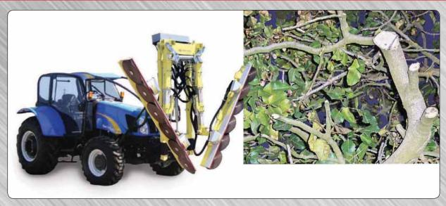
An almond grower who purchased a COLLARD Tree Hedger states: "The COLLARD Tree Hedger has larger diameter cuts than any sickle machine, less maintenance, and fewer moving parts. The blades throw much of the brush into the row instead of dropping into the tree canopy. The COLLARD Tree Hedger is more convenient - able to cut how you want and use a smaller tractor that has a lighter "footprint" in the field."
