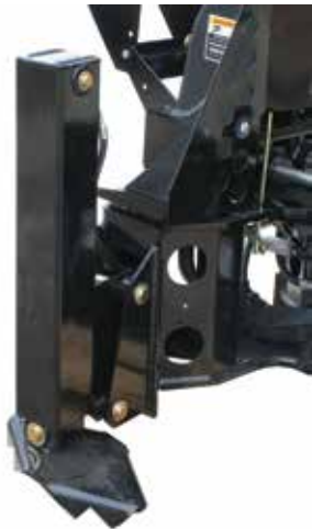
Vertical Stabilizer Assembly
