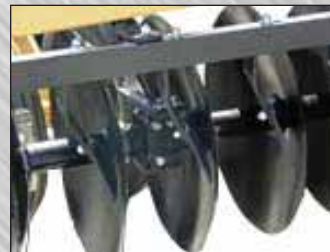
1 1/2" Triple sealed bearing in cast trunnion mount housing
