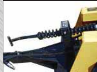
Self leveling, spring cushioned hitch with hand crank
