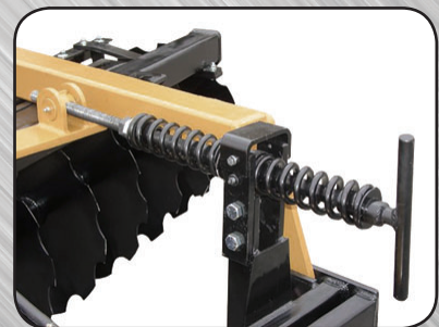
Self leveling spring cushioned with hand crank
