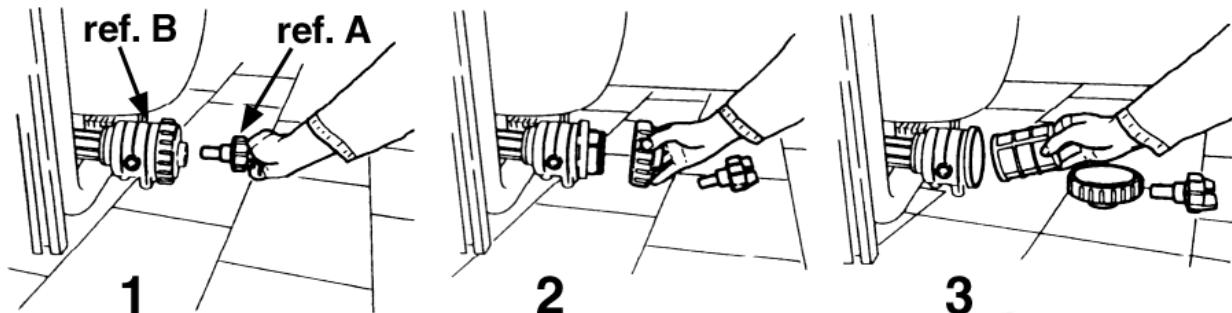
1. Remove the plunger valve (ref. A) from filter assembly (ref. B).
